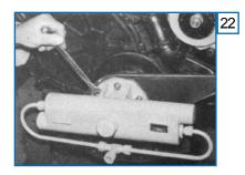
22. Fit starter unit to the engine.
