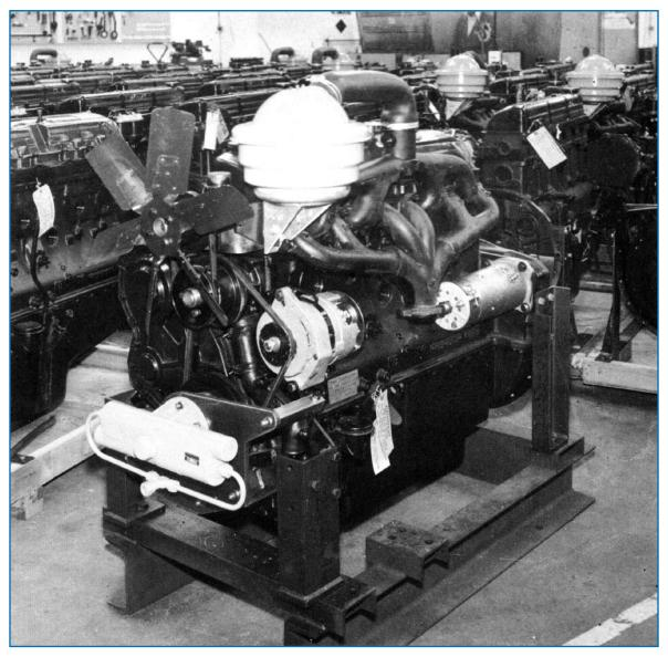
Diesel Engine with Handraulic Starter fitted.
