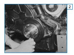
2. Fit engine dog adaptor to crankshaft pulley.
