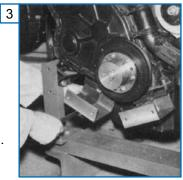
3. Fit two mounting brackets to the engine.
