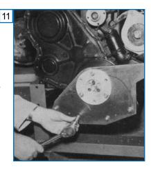
13. Refit alignment tool in a new position to overcheck ease of fitting / squareness / concentricity. If problems arise, re-check earlier shim arrangements and adjust as necessary. When alignment tool fits easy, proceed.
