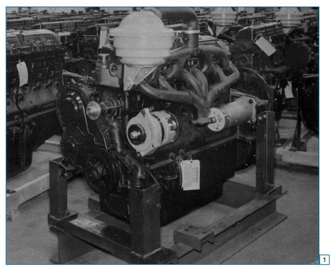
Diesel engine ready to receive Handraulic Starter.
