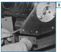
8. Check gap between mounting bracket and plate. Use two 0.049 inch / 1.25 mm thick shims (18SWG) to accommodate extreme tolerances.
