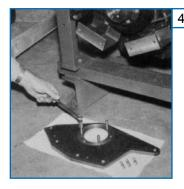
4. Fit three of the six studs to the mounting plate as shown.
