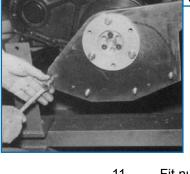
11. Fit nuts and washers to studs and tighten. Also tighten bolts holding engine brackets to engine.
