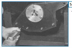
With alignment tool re-assembled, drill two dowel holes.
